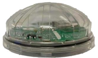
The Luminext OLC400 Zhaga Wirepas is a product in the Luminext program for dynamic dimmable street lighting with remote management. The OLC400 Zhaga Wirepas is suitable for fixtures with a Zhaga connector and D4i driver. The OLC400 Zhaga Wirepas controllers automatically forms a wireless-sensor-and-control network that is self-organizing and self-synchronizing in combination with other OLC400's and a RF4 gateway.
