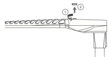
2. Connect OLC400 Zhaga Wirepas to the connector and twist to lock in place
