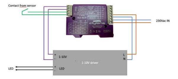
Connect the power input of a 1-10V driver to the 230V output of the OLC154. Contacts 3 and 4 can be used to connect a potential free contact from a motion sensor, PIR or Radar.
