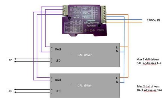
Connect the power input of a DALI driver to the 230V output of the OLC154.
