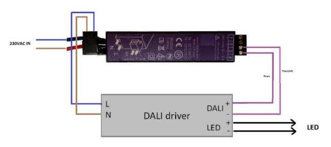
Connect the power input of a DALI driver to the 230V output of the OLC150.
