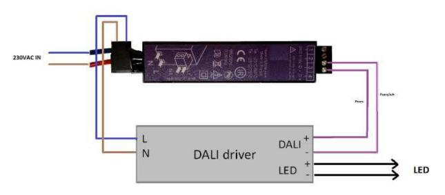
Connect the power input of a DALI driver to the 230V output of the OLC150. Contacts 1 and 2 can be used to connect a potential free contact from a motion sensor, PIR or Radar.
